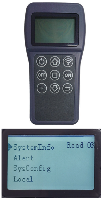
Fig. 5.1a Solar panel remote control & LCD
