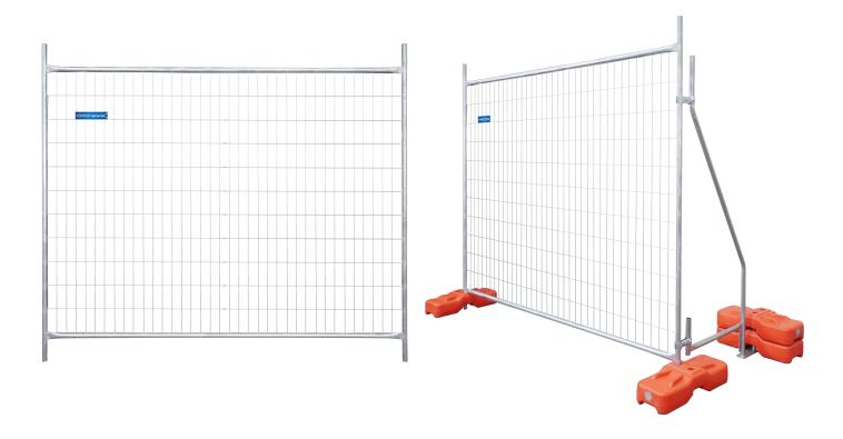
Our temporary fencing panels provide a sturdy, durable, and portable solution for securing construction sites, events, and other areas that require temporary enclosure. 2000 Series Heavy Duty is an evolution of the 2000 Series temporary 32mm OD fence panel with 2mm wall thickness and 4mm wire mesh for extra durability.
